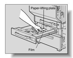
**3** Slide the lateral guides to fit the size of paper to be loaded.
